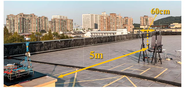
Fig. 7. Experimental setup used to study the impact on communication link performance of MG's vorticity.
