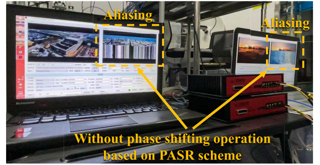
Fig. 18. Without the phase shifting operation based on the PASR scheme, the channel isolation will cease to exist, and the multiplexed video signals are going to be aliased.
