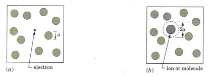
Figure 2.6 Geometry for mean-free-path calculation showing a particle traveling into the plane of the drawing and encountering gas molecules of diameter a; the particle is an electron in part (a) and an ion in (b).
