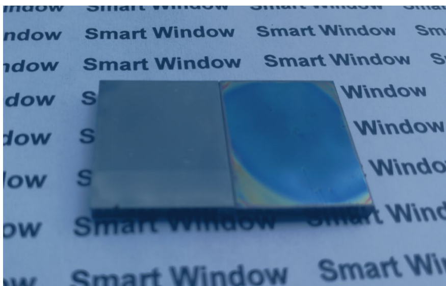
Figure S6. Photographs of the pure perovskite film (left) and the perovskite film covered by \text{VO}_2 layer (right) on PTAA-coated ITO substrates.
